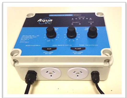
The 2 nd outlet is designated "AUX" is specifically designed for dosing pump.
